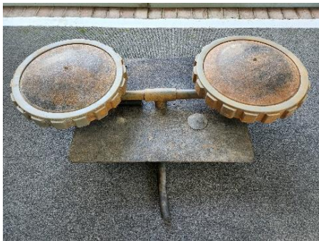
Old diffuser (installed in 2005 and removed in 2022)
